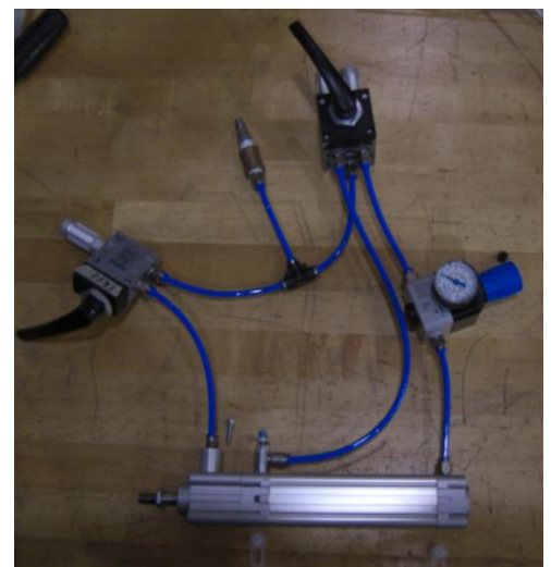
Figure 3: Schematic (left) of pneumatic system showing all key components except the load cell at the end of the pneumatic rod. Not to scale. Photograph (right) of the layout and connections of the constructed pneumatic system after verification of basic performance.
