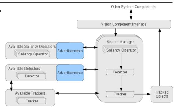
architecture of the vision system for online learning of new object detectors combining available saliency operators and feature detectors
