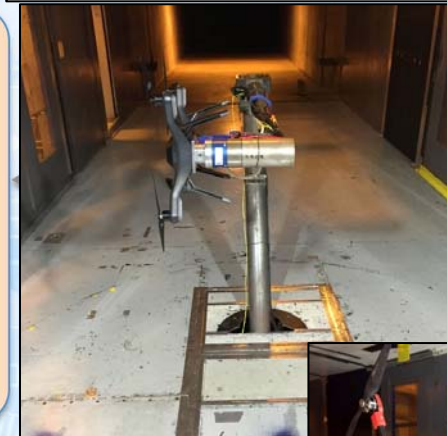
Multi-Copter Wind Tunnel Test
