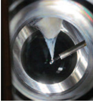
Boron nitride nanotube grown in the NIA BNNT chamber.
